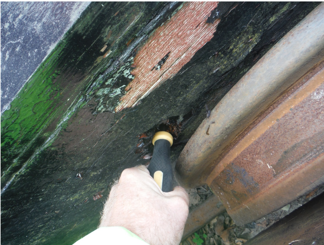
Decay timber of beam MB3 near back wheel
